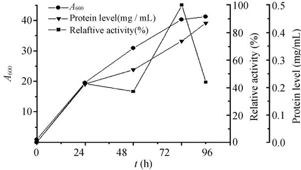
Fig. 3 Expression of transformed *P. pastoris* GS115/pPICZαA-man'. Cultured under 28°C, induced with 1% methanol, re-*at*MAN47 was highly active after induction with methanol for 72 h and has activity of 1.067 U/mL, and the yield was 440 mg/L.
