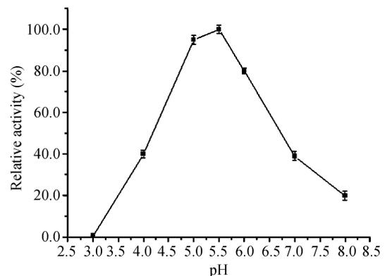
Fig. 7 Effect of pH on the activity of purified re-*at*MAN47. The optimal pH was obtained by incubating the enzyme at 60°C for 30 min at different pH. To adjust the pH range, 0.2 mol/L Na<sub>2</sub>HPO<sub>4</sub>-0.1 mol/L citric acid buffer was used for pH 3.0–5.5; 0.2 mol/L Na<sub>2</sub>HPO<sub>4</sub>-0.2 mol/L NaH<sub>2</sub>PO<sub>4</sub> buffer was used for pH 6.0–8.0. After the incubation period, the enzyme activity was assayed by the DNS method.
